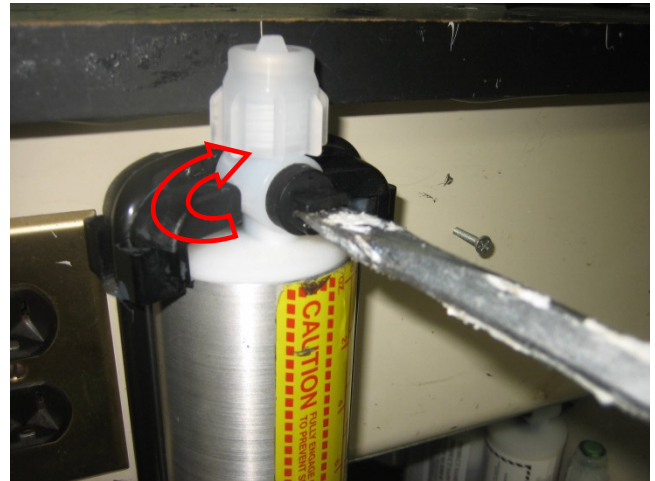
Step 6 – turn ball valve 90 degrees into open position
