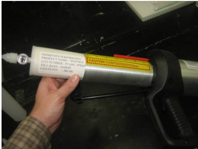
Step 1 - insert cartridge (CTG) into SX gun
