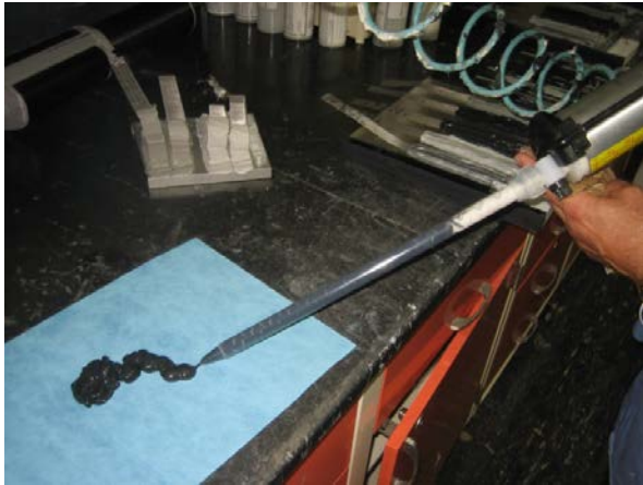
Step 13 – dispense ~80 ml of material prior to using in application
