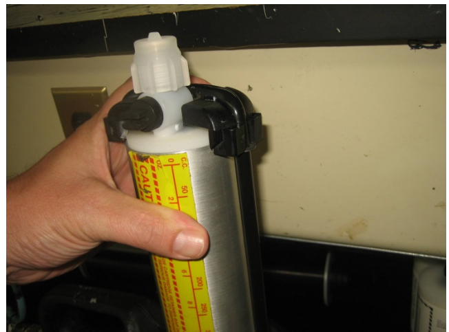
Step 4 – snap retainer yoke closed
