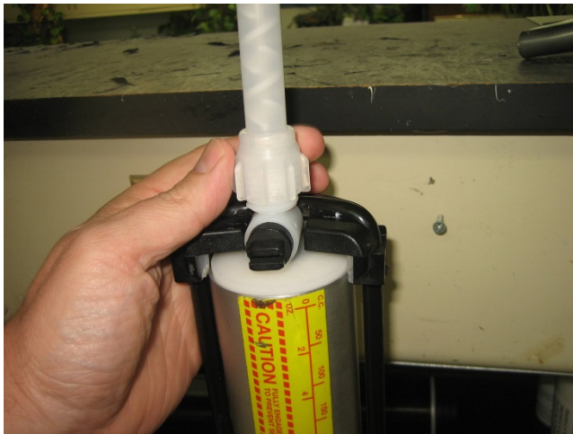
Step 11 – fasten static mixer to CTG with retaining nut
