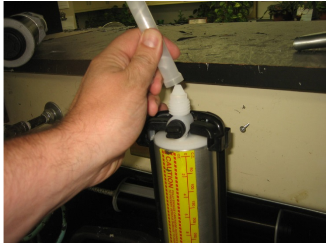
Step 10 – place static mixer onto CTG
