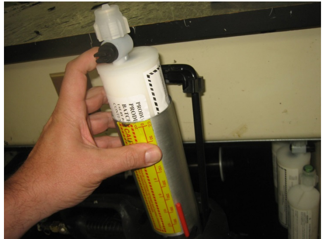
Step 2 – push CTG fully into gun cylinder
