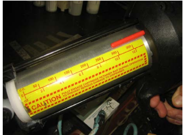
Orange indicator should be near 300ml prior to using material
