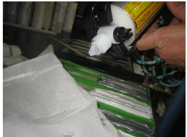
Step 8 – squeeze trigger briefly (over container) until both parts A&B are exiting the CTG
