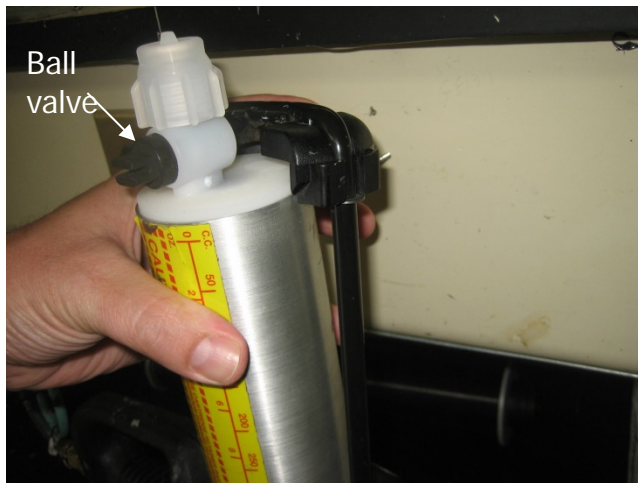
Step 3 – line up ball valve with retainer yoke
