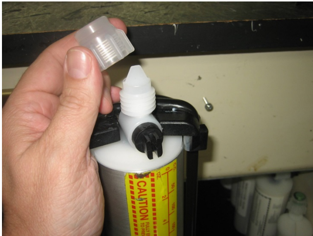
Step 5 – remove retaining nut
