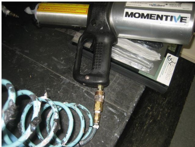
Step 7 – connect to air source
